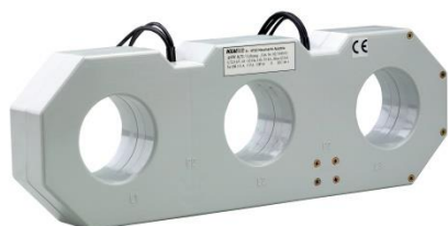
Current transformer type JW 11/02 in a three-phase slide-in design. Inner diameter of holes 75mm. Dimension between holes 150mm.
